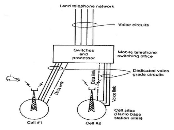
a mobile unit, a cell site, and a mobile telephone switching office (MTSO)
